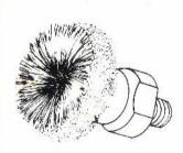
T.B. BRUSH. This design of brush is used mainly for light brushing and polishing of tube surfaces in all types of tubular plant and is particularly useful for CURVED tubes. Two types are available, i.e. LIGHT pattern filled with 32/33g or 30g FINE wire and HEAVY pattern (in larger hubs containing more wire) filled with 27g crimped wire. Made in all sizes between 12 mm and 76 mm diameter in the LIGHT pattern and 38 mm to 102 mm diameter in the HEAVY pattern.
