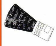
S.H.K. BRUSH. This brush has a very strong scouring action indeed and is much in demand by some Sugar Mills. Rapidly cleans and polishes all types of STRAIGHT tubes leaving an excellently burnished surface. It is filled with 20g crimped wire as a standard. Available in tube sizes 22 mm to 102 mm internal diameter.
