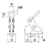
NB: The angle between the chain / rope legs must not exceed 90° (45° from vertical).
